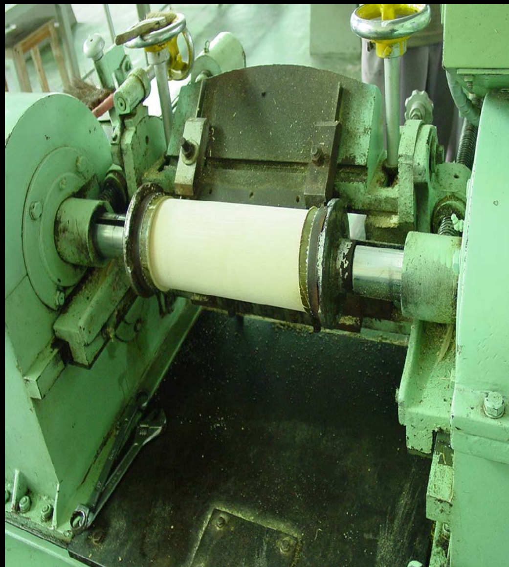
Bamboo veneer by rotational peeling
