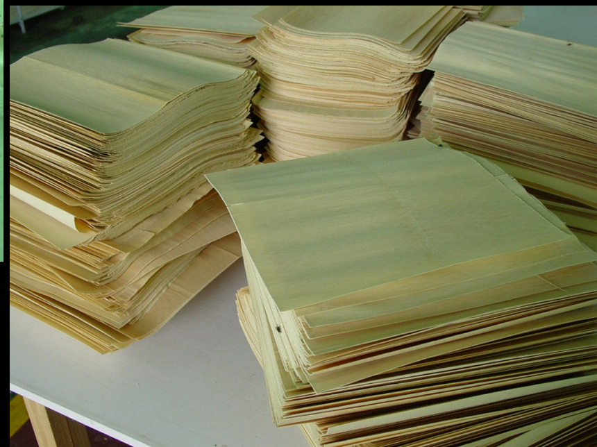
Bamboo veneer by rotational peeling
