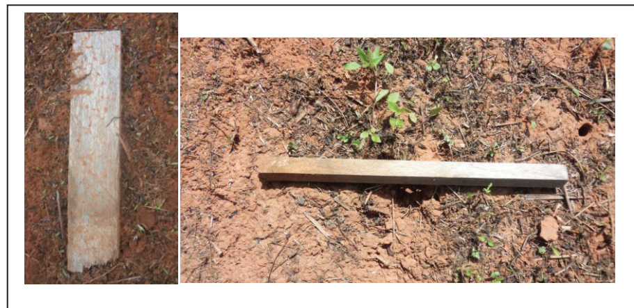
Figure 4. Rejected 0.4x3.8x25.4 cm. and 1.9x1.9x45 cm. Ai sample sizes
