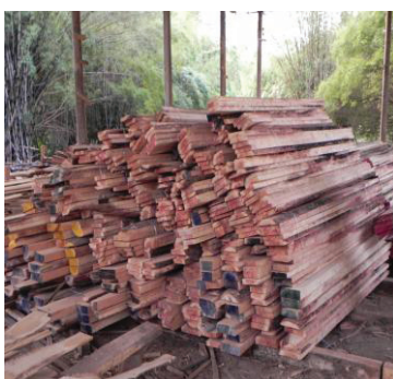
Figure 1-3 Neem logs process and stack for test.
