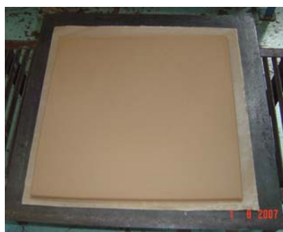
Figure 4 Medium Density Fiberboard from Acarcia crassicaarpa .
