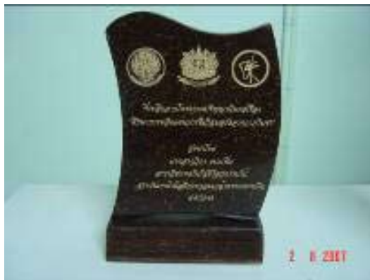
Figure 4. Sample product of particleboard from tea leaf wastes.
