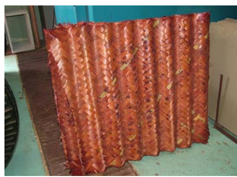
Figure 9. Undulation roof form bamboo-mat.
