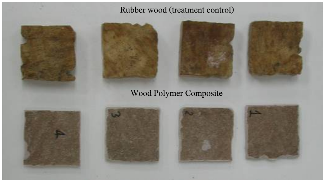
Figure 17. Fracture of Wood Polymer Composite and rubber wood (treatment control) by termite.
