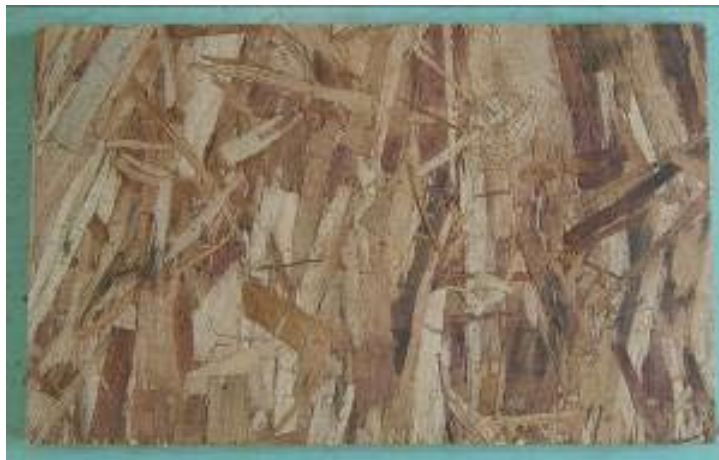
Figure 5. Oriented Strand Board (OSB) from Eucalyptus camaldulensis .
