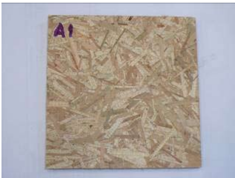
Figure 10. Sample particleboard form leaves of cat-tail.
