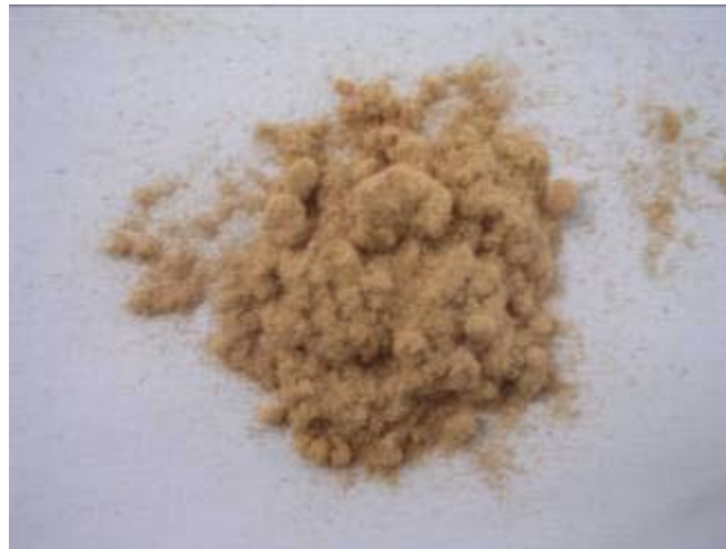
Figure 4. Rubber wood fiber character from Thermo-mechanical pulp
