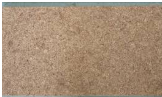
Figure 4. Sample particleboard form agricultural waste .(bagasse, fiber of costusroot palm , bark of Corn and corncob )
