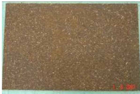
Figure 5. Particleboard from bark of Eucalyptus camaldulensis
