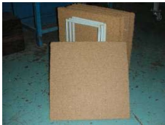
Figure 4. Sample of thermal insulation form natural agricultural wastes.
