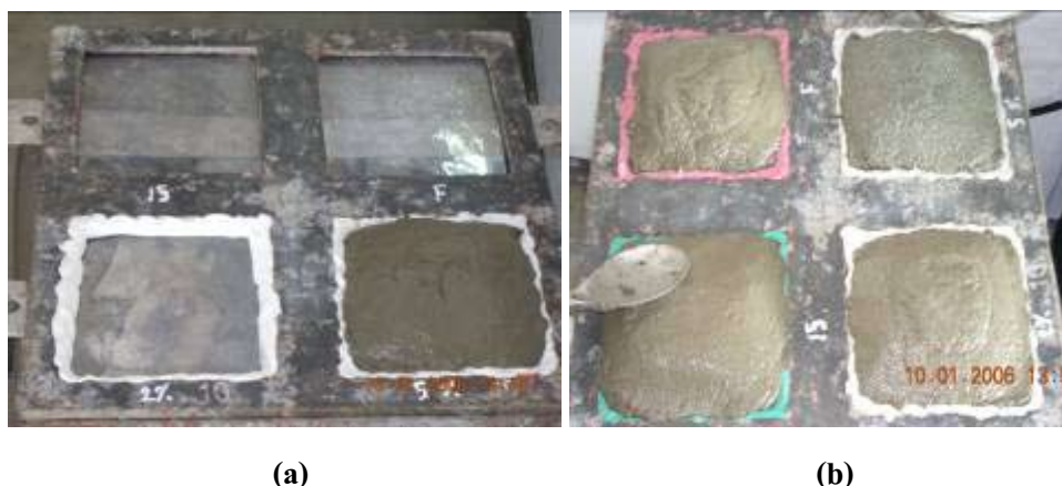
Figure 3. (a) The model metal of cement-boards. (b) Preparing to board making.
