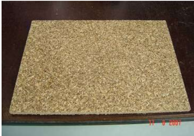
Figure 4. Particleboards make of physic nut stem.
