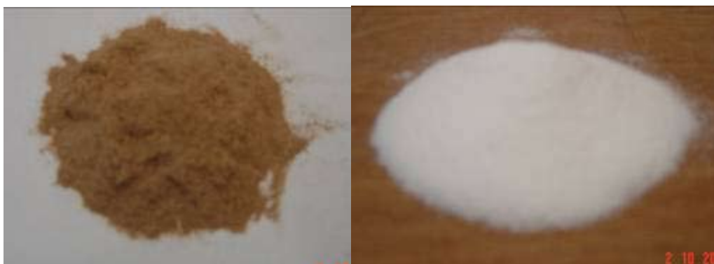
Figure 2. Medium Density Polyethylene ( MDPE ) and particles of Acacia crassicaarpa before board making.
