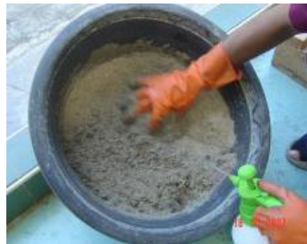
spray 1 % \text{CaCl}_2 solution
