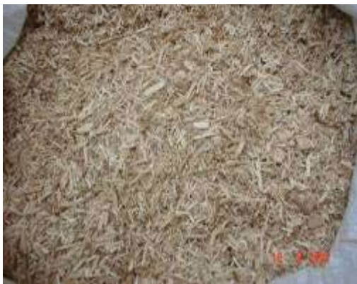
Wood particles after Hammer mill and Screening
