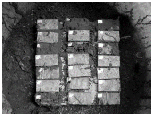
Figure 3 Damage on wood composites in field test.
