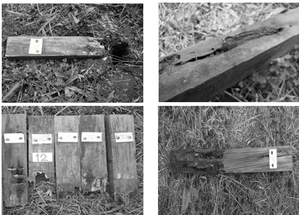
Figure 2 Failure of P. caribaea specimens in field testing for natural durability.
