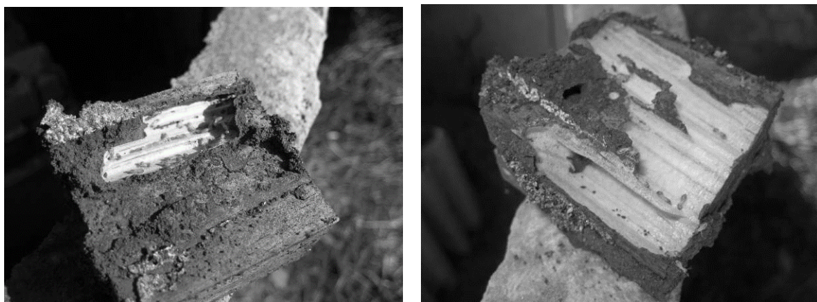
Figure 4 Pinus caribae specimens after 10 months of exposure.
