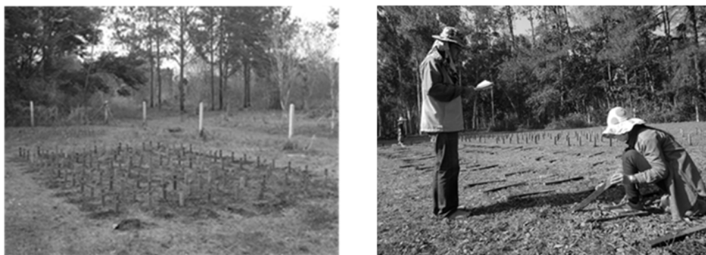
Figure 1 Natural durability testing and periodic inspection of treated P. caribaea .
