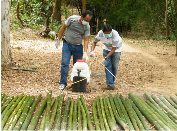
Figure 13 Wood preservative spraying.
