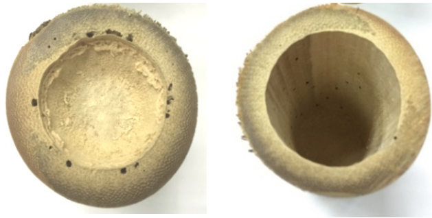
Figure 11 Thyrsostachys oliveri Gamble was treated by water. (Control)
