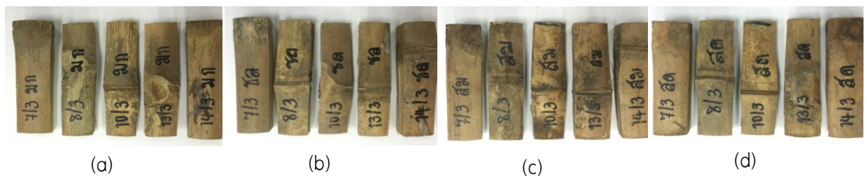
Figure 5 Bambusa beecheyana Munro was treated by soaking in plant extracts solution of (a) Abrus precatorius Linn., (b) Lepisanthes fruticosa , (c) Ageratina adenophora , (d) Azadirachta indica . There was no damage after 12 months exposed to powder-post beetle in laboratory.
