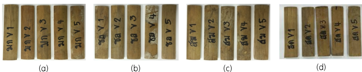
Figure 8 Dendrocalamus copelandii (Gamble ex Brandis) was treated by Pressure Treatment, using plant extracts solution of (a) Abrus precatorius Linn., (b) Lepisanthes fruiticosa , (c) Ageratina adenophora , (d) Azadirachta indica . There was no damage after 12 months exposed to powder-post beetle in laboratory.
