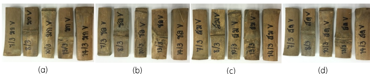
Figure 6 Bambusa beecheyana Munro was treated by Pressure Treatment, using plant extracts solution of (a) Abrus precatorius Linn., (b) Lepisanthes fruiticosa , (c) Ageratina adenophora (d) Azadirachta indica . There was no damage after 12 months exposed to powder-post beetle in laboratory.
