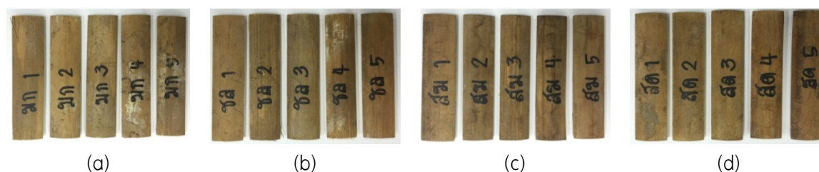
Figure 7 Dendrocalamus copelandii (Gamble ex Brandis) was treated by soaking in plant extracts solution of (a) Abrus precatorius Linn., (b) Lepisanthes fruiticosa , (c) Ageratina adenophora (d) Azadirachta indica . There was no damage after 12 months exposed to powder-post beetle in laboratory.
