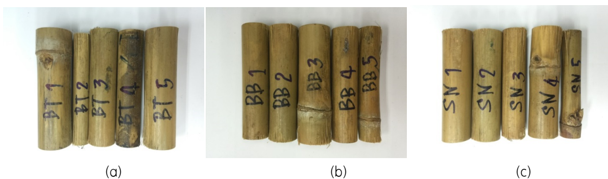
Figure 3 Thyrsostachys siamensis Gamble was Treated by soaking in plant extracts solution of (a) Melia azedarach , (b) Chromolaena odorata , (c) Stemona collinsae . There was no damage after 12 months exposed to powder-post beetle in laboratory.
