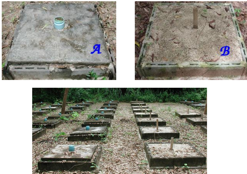
Fig.2 Plots of termiticides test (A) MGB (B) ST
