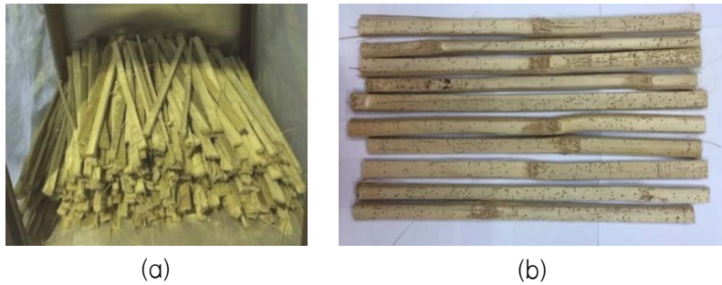
Figure 12. Powder-post beetle rearing bamboo sticks for infestation testing (a) Before testing (b) After 12 months testing
