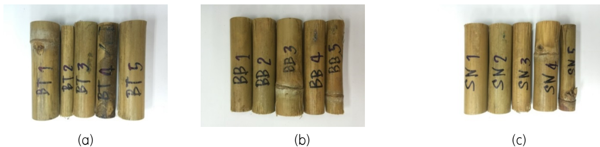
Figure 3. Thyrsostachys siamensis Gamble was Treated by soaking in plant extracts solution of (a) Melia azedarach , (b) Chromolaena odorata , (c) Stemona collinsae .
