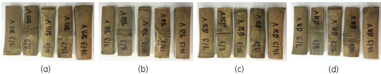
Figure 6. Bambusa beecheyana Munro was treated by Pressure Treatment, using plant extracts solution of (a) Abrus precatorius Linn., (b) Lepisanthes fruiticosa , (c) Ageratina adenophora (d) Azadirachta indica . There was no damage after 12 months exposed to powder-post beetle in laboratory.
