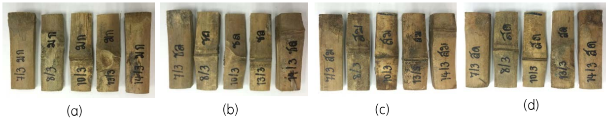
Figure 5. Bambusa beecheyana Munro was treated by soaking in plant extracts solution of (a) Abrus precatorius Linn, (b) Lepisanthes fruiticosa , (c) Ageratina adenophora (d) Azadirachta indica . There was no damage after 12 months exposed to powder-post beetle in laboratory.
