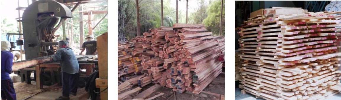
Fig. 3 Neem logs process and stack for test.
