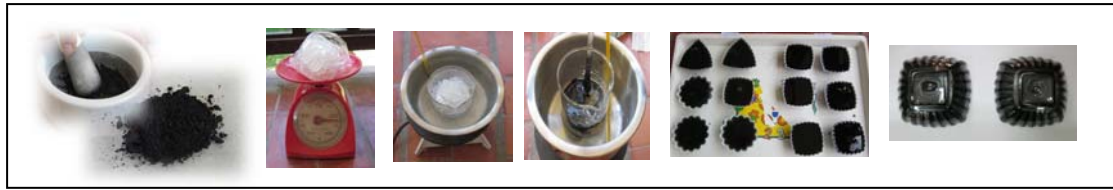
figure 2. Charcoal soap making from Activated carbon
