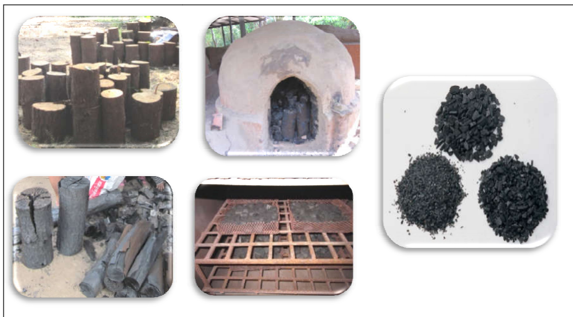
Figure 1 Methods of activated carbon preparation from Pinus spp.
