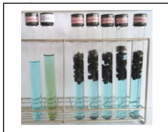
Figure 8 Comparative activated carbon from Pinus spp. utilization with food color water and EM (2.0)
