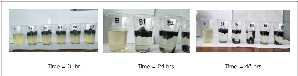
Figure 13 Comparative activated carbon from Pinus spp. utilization with EM and waste water in front of factory in Samutsakorn province
